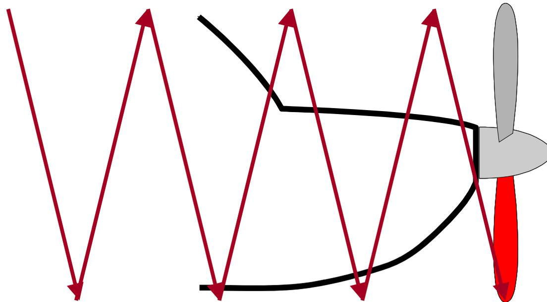
How the blade tip travel produces the **HELIX ANGLE**
