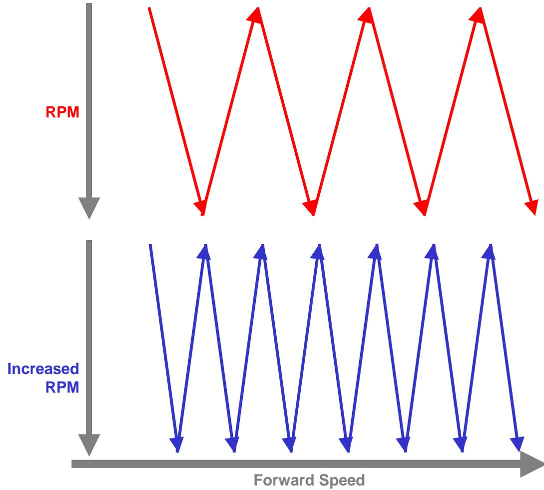
How an increase in RPM changes **HELIX ANGLE**
