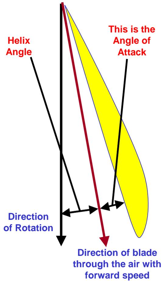
How lift is produced by a Propeller Blade
