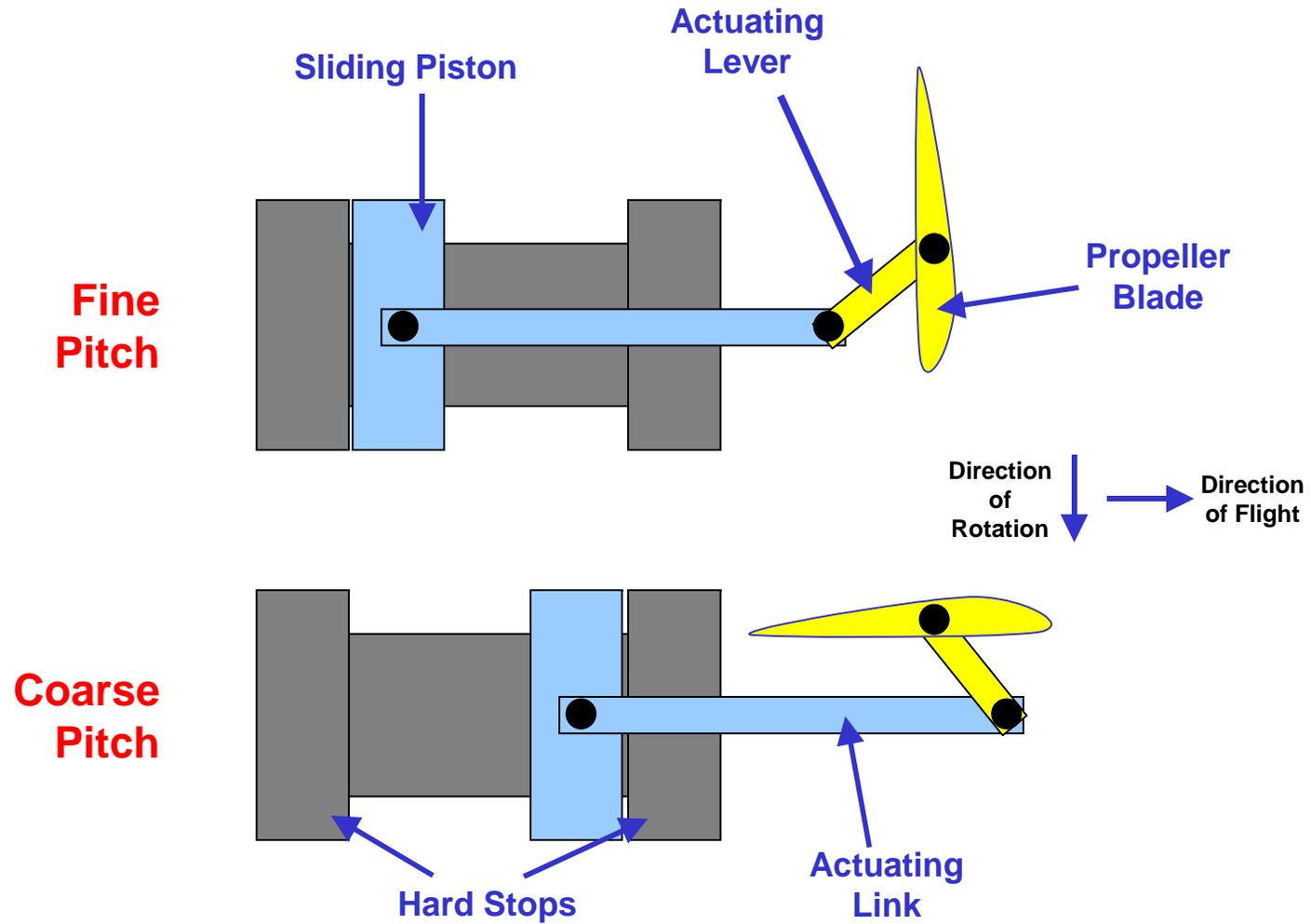
All propeller blades are actuated by the same mechanical linkage
