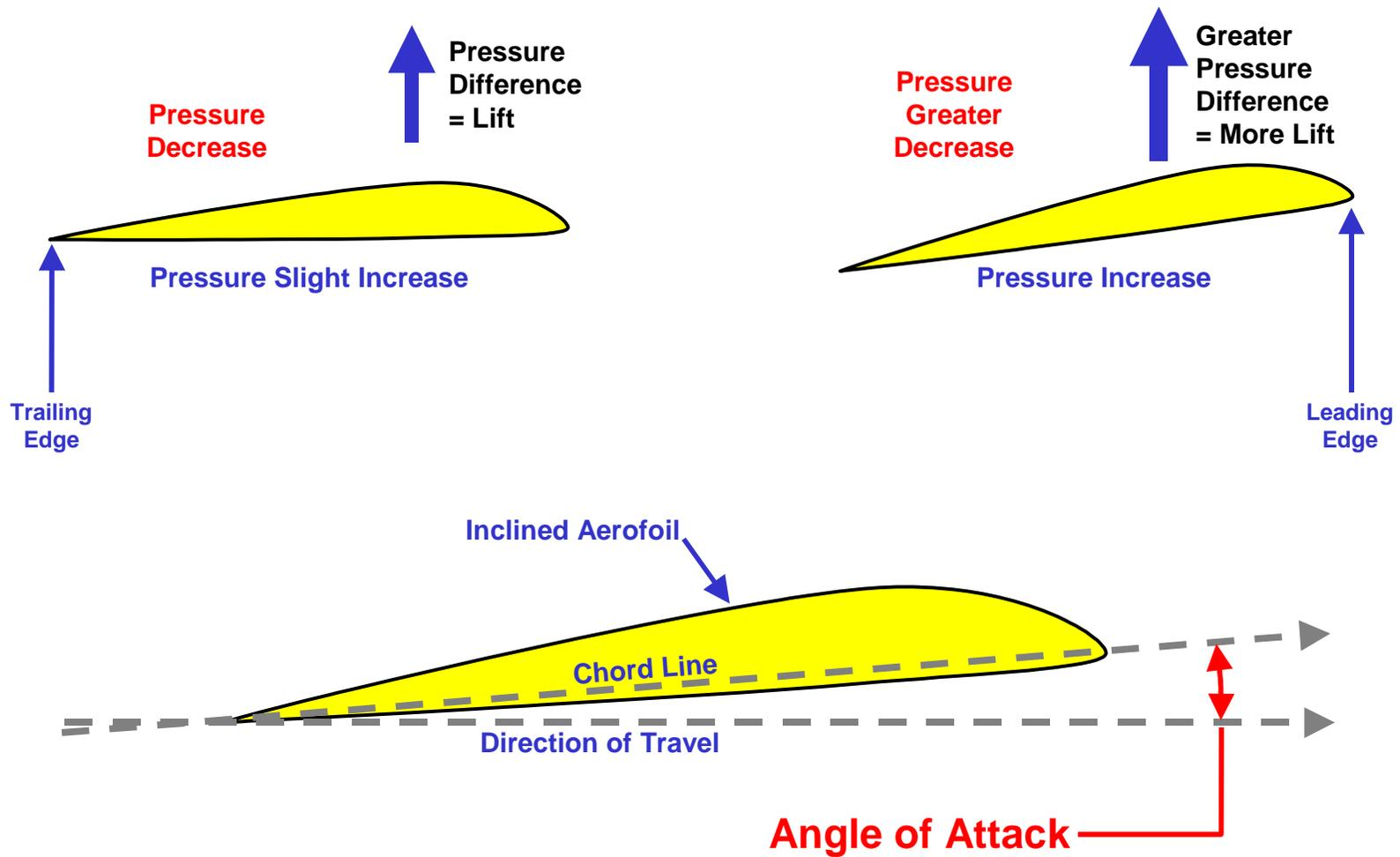
How lift is produced by a Wing
