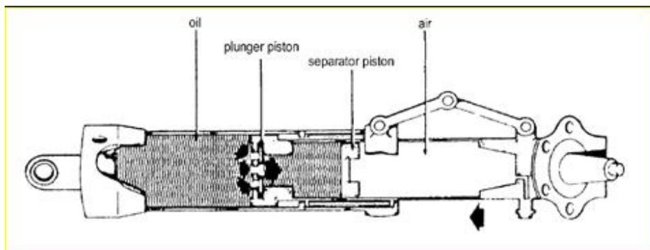
The gas or oil will stay slightly compressed when it has the weight of the aircraft on it, so it provides the aircraft with a cushion against bumps whilst taxiing.
