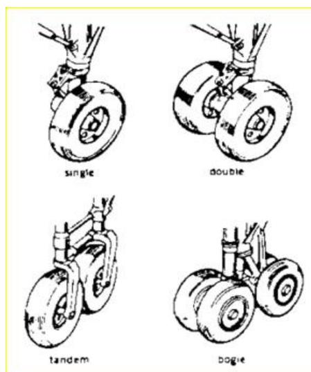
As aircraft become heavier, the loading on a single wheel increases, leading to a great increase in the damage done to runways.
