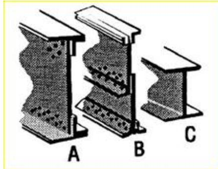
A & B are made of sections fastened together, but some modern aircraft would have the spar made from a single piece of metal, as in C, making it stronger and lighter.
