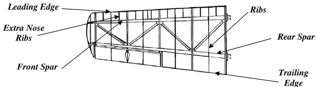
37. Attached to the front spar is the leading edge section, in this case it is made up of nose ribs and the leading edge itself.
