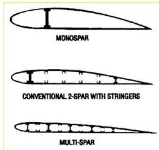
For example, supersonic aircraft, such as the Eurofighter Typhoon, require extremely thin wings, and hence use a multi-spar layout.
