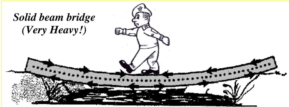
*The effect of a weight on a solid beam bridge*
