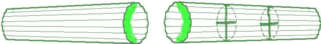
We can do the same with the structure of the bridge, and use even thinner walls, provided they are properly braced to withstand the loads.
