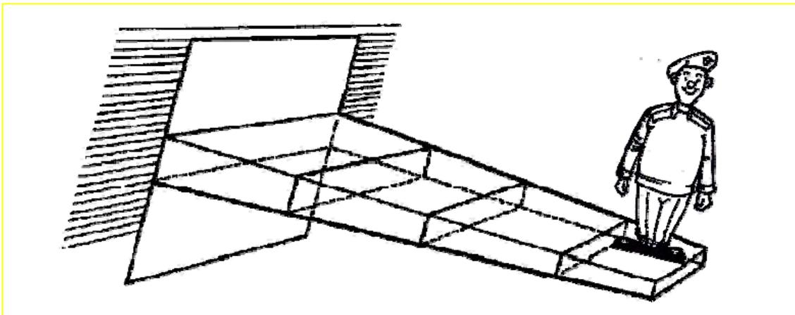
The cantilever structure is widely used in aircraft, because airframe design contains many structures which are attached at one end. The wings are just one example of this.
