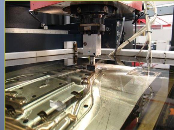
The material removal from the workpiece occurs by a series of rapidly recurring current discharges between two electrodes, separated by a dielectric liquid and subject to an electric voltage.
