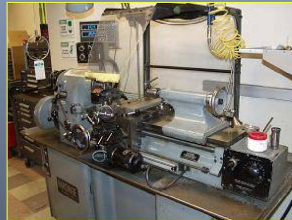
Turning machines can be used to enlarge drilled or cored holes – this process is referred to as '*Boring*'.
