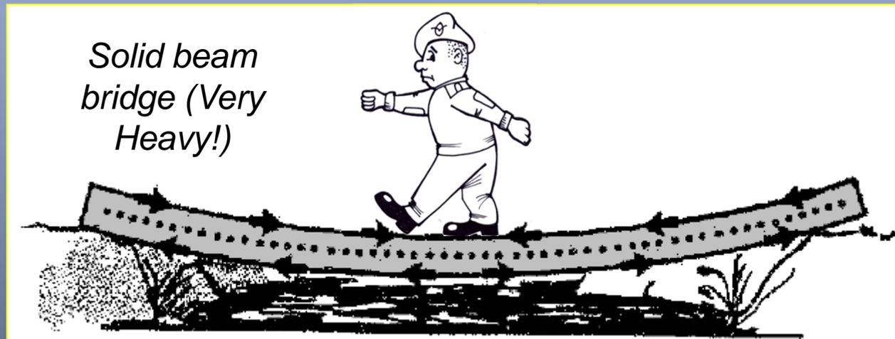
*The effect of a weight on a solid beam
